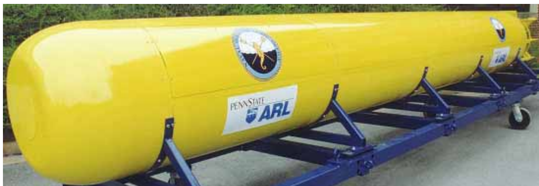
Fig.06: ARL/Penn State University fuel cell UUV “Seahorse”. Source: ARL
