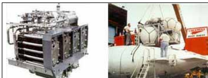
Fig.26: 10kW PEM prototype for undersea vehicle (1990) and 30kW alkaline fuel cell unit for UUV (1980). Source: UTC Fuel Cells
