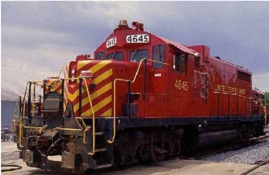
Fig.15: 1.2MW PEM locomotive. Source: Fuelcell Propulsion Institute.
