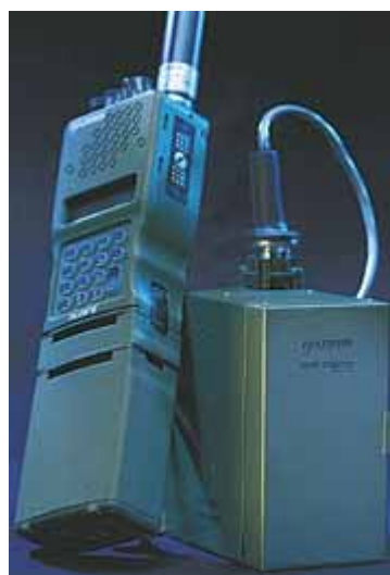
Fig.21: MTI DMFC power source. Source: MTI.
