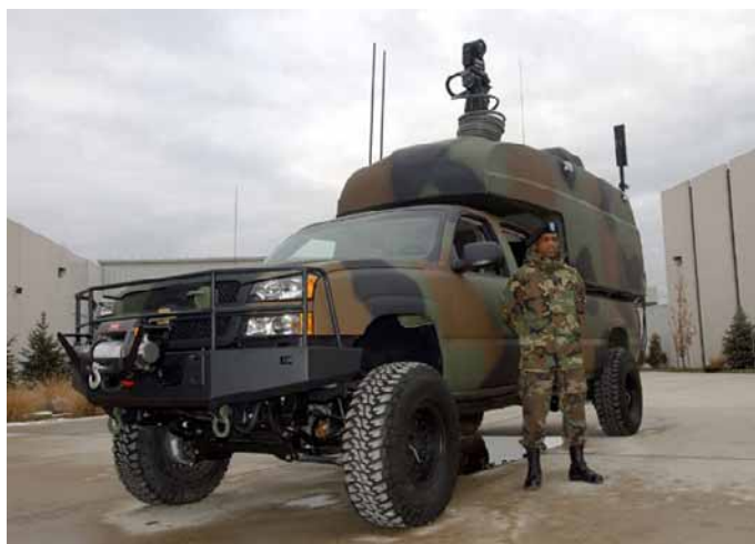
Fig.18: GMD pickup with 5kW APU fuel cell. Source: General Motors
