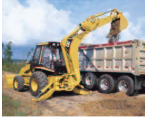
Figure 3.1 The hydraulic backhoe extends the strength and reach of its human user using high pressure hydraulic actuators.
